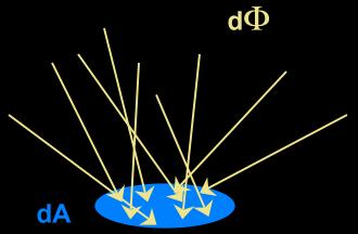
Irradiance: power per unit area falling on a surface.
